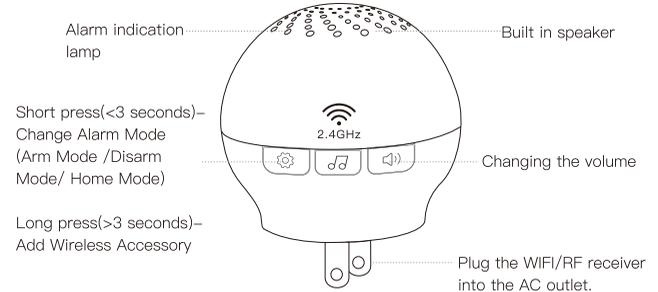
Arm Mode/Home Mode: Any alarm device will trigger alarm.
